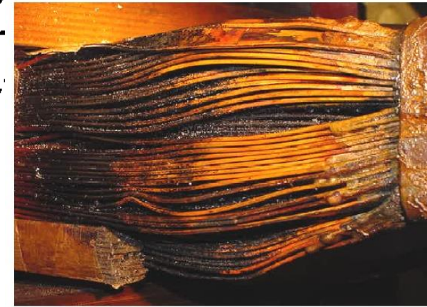
Station 3 Gen. Transformer 5 overheating
