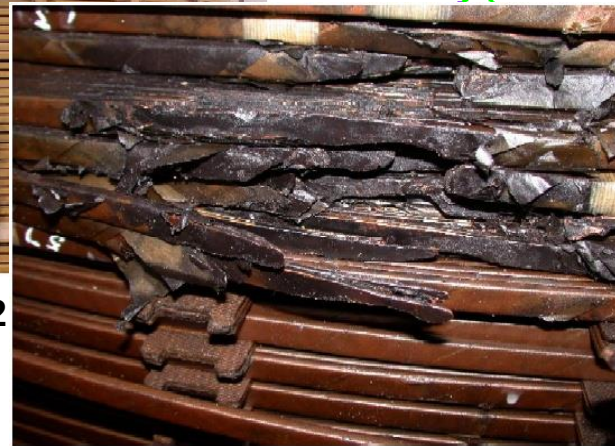
Station 3 Gen Transformer 4 damage
